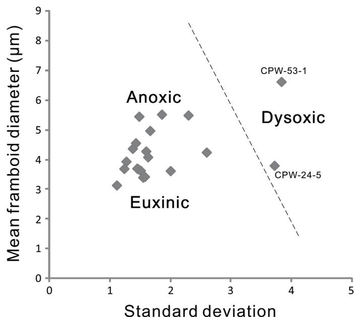
**Figure 3.** Cross-plot diagram showing mean diameter (M) vs. standard deviation (SD) of pyrite framboid sizes from the West Pingdingshan section. For determination of the dash line separating euxinic/anoxic facies from dysoxic facies, see text (after L. Tian et al., 2014). Note that all samples fall into the anoxic-euxinic field, except for CPW-24-5 (end-Dienerian) and CPW-53-1 (early Spathian), which fall into the dysoxic condition field.
